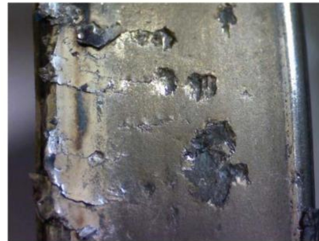
Rail Disc Surface after 200 000 cycles, Severe Spalling
