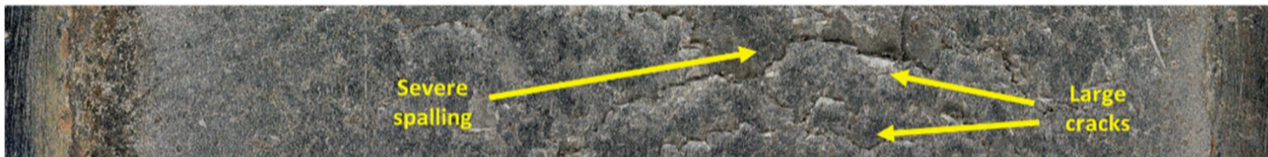
TOR Lubricant in Wet Conditions (25 000 cycles, pre-existing cracks)
